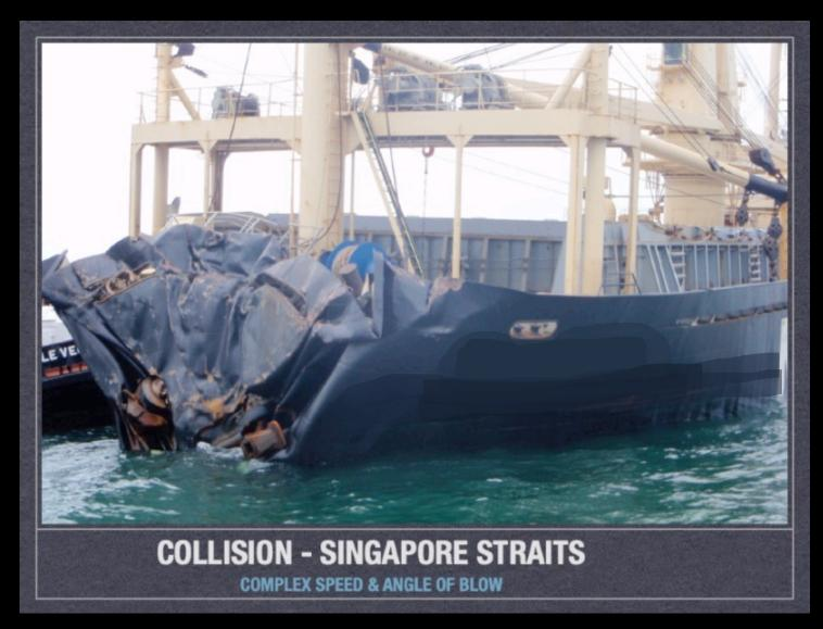
The smaller ship, crossing the Singapore Traffic Separation Zone, was the give-way ship & altered to starboard.
